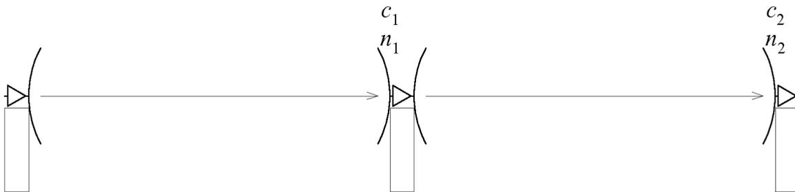
$C_1$  is the carrier power at the output of the first link. It is amplified by an amplifier, then undergoes gains/losses associated with a standard radio link to the next hop. The cumulative gain between the links is defined as  $\alpha$ , so that the output signal power is  $C_2 = \alpha C_1$ .
